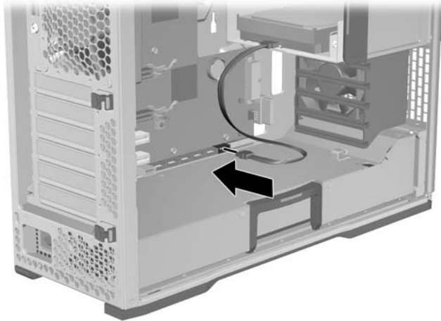
Figure 5-35 Connecting the data cable to the system board
