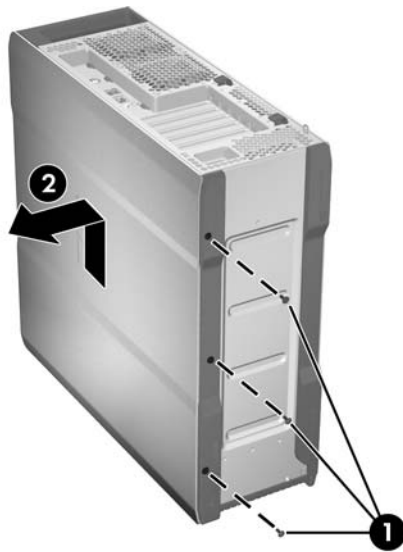
Figure 5-6 Removing the right side panel
