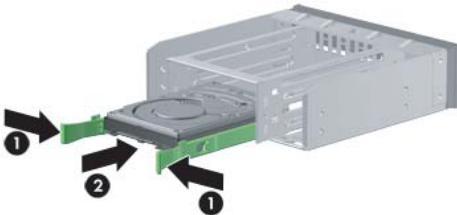
Figure 5-63 Installing the drive in the optical bay bracket
