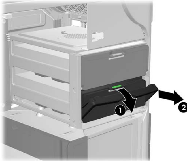
Figure 5-36 Removing the drive from the chassis
