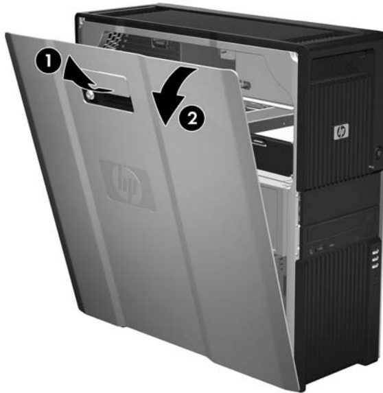
Figure 5-3 Removing the side access panel
