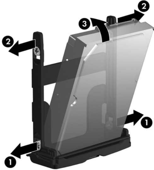
Figure 5-39 Installing the drive in the carrier
