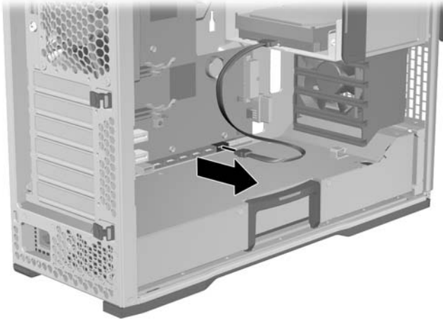
Figure 5-41 Disconnecting the data cable from the system board
