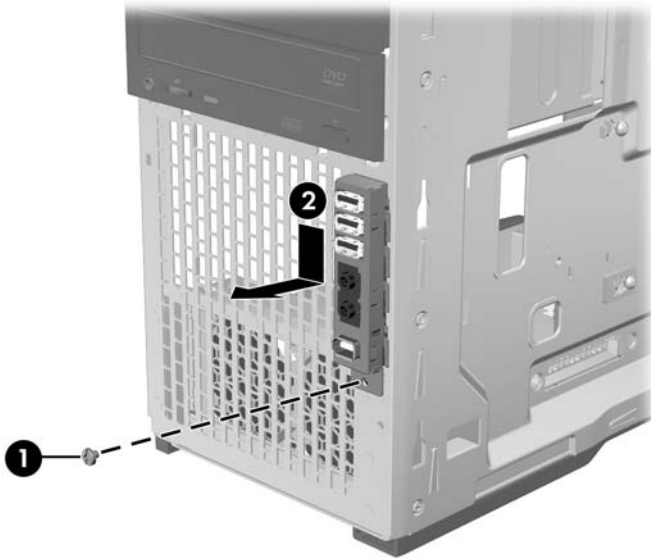
Figure 5-14 Removing the front panel I/O cable assembly
