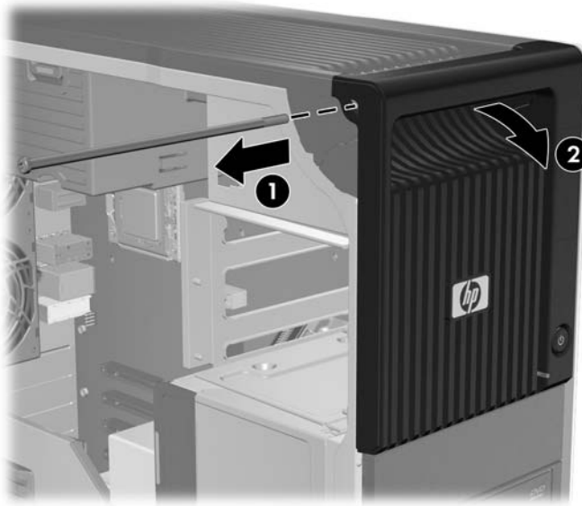
Figure 5-11 Removing the upper front bezel
